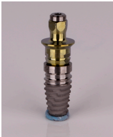
Fig. 4. Hybrid design titanium implant with smooth, machined surface of the coronal portion and a plasma-sprayed surface of the apical portion of the implant in one body.
