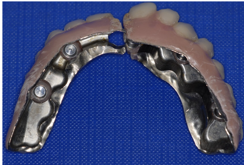
Figure 3. Prosthetic failure: A prosthesis fracture occurred after 16 months due to a design error in the original framework (Patient no. 1). The load-bearing connector area had been designed too thin/narrow, as determined in a retrospective analysis.
