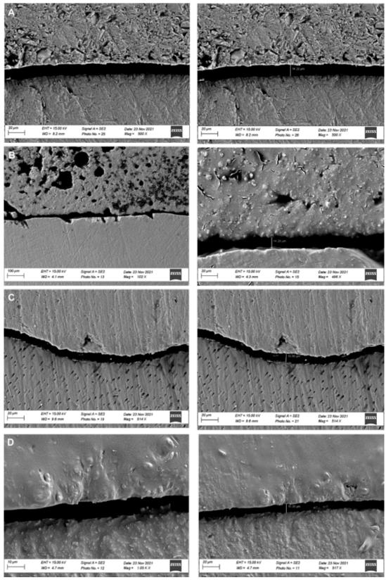
**Figure 5.** Representative SEM microphotograph of material-dentin interface. (A) Filtek<sup>TM</sup> Z350 XT, (B) Biodentine<sup>TM</sup>/ Filtek<sup>TM</sup> Z350 XT, (C) Cention N<sup>TM</sup>, and (D) Activa<sup>TM</sup>.
