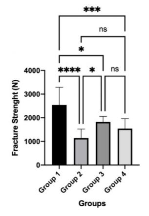
**Figure 1.** Means and standard deviations for fracture resistance loads (N) \*Indicate statistical differences between groups.
