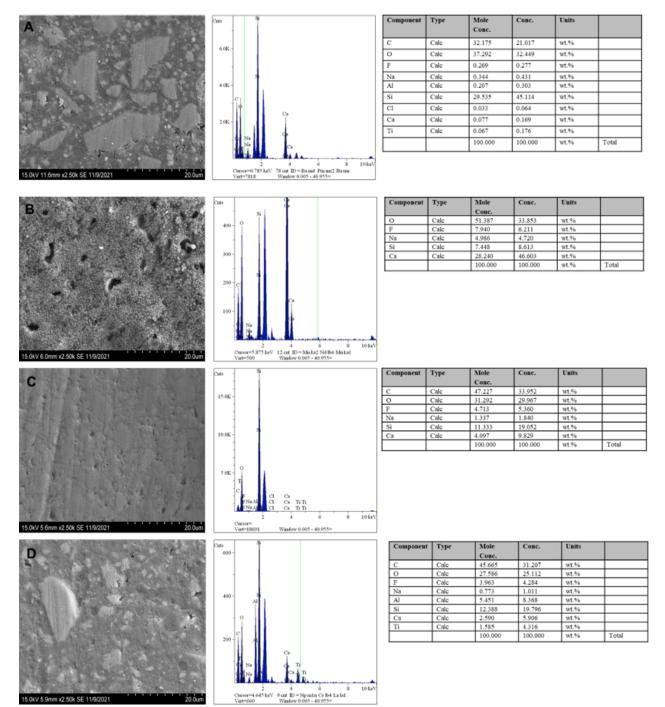
Figure 4. EDAX spectrum for (a) Filtek™ Z350 XT, (b) Biodentine™/ Filtek™ Z350 XT, (c) Cention N™, and (d) Activa™.
