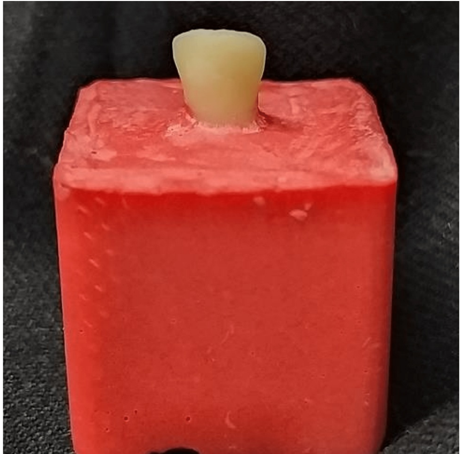
FIGURE 2: Tooth placed in an acrylic cube.
